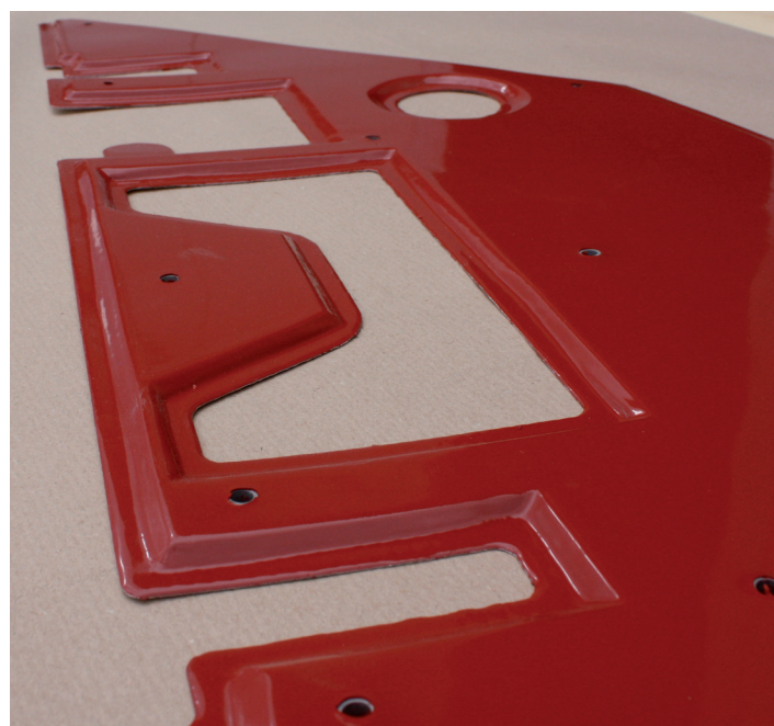
Structural part of helicopter with high temperature insulation coating under topcoat
